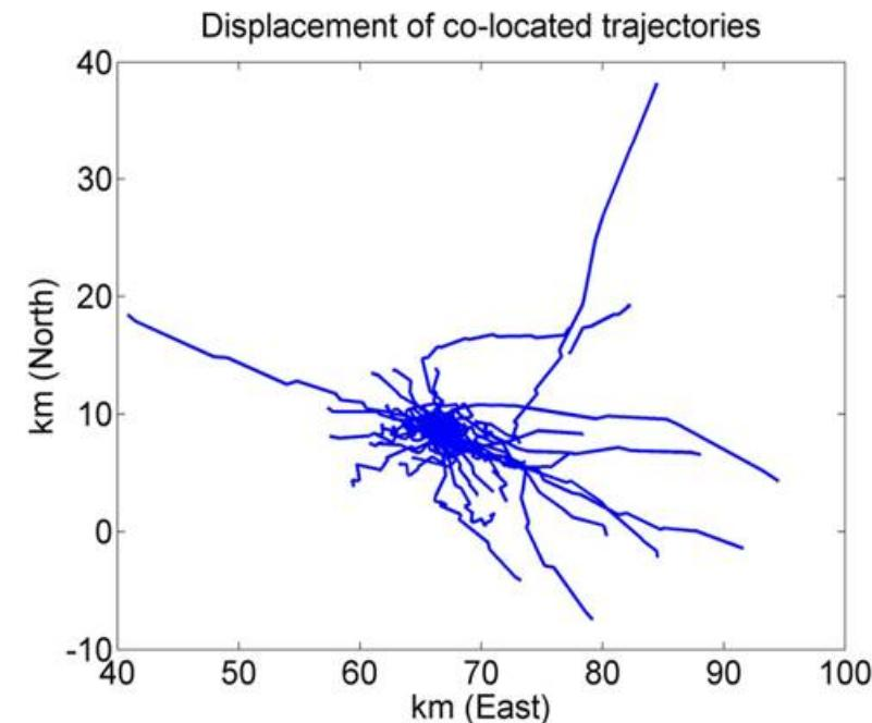
The displacement of collocated trajectories is given by the difference of positions for two collocated instruments at the same altitude. X axis is distance along parallels and Y axis along meridians. Distance range is 45-95 km.
